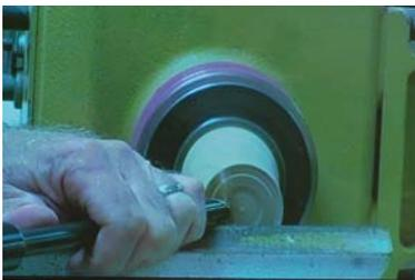
The project is a clam box: two thin curved pieces, pierced, and fit together. He recommended Golden airbrush paint as it doesn't clog the brush. To do this project he rounded a piece of maple. Then he started to concave the end of the blank using a draw cut. One can make it any depth desired.
