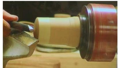
Jerry used a saw to complete the parting as this eliminates the possibility of the wood tearing. Then using the parting tool cut the edge of the piece still in the chuck till the rabbit fits on securely. He sands starting about 220 grit and goes to 400.
