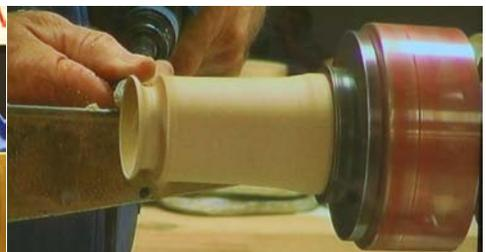
He uses a depth gauge preset to the depth he wants. The turning is finished using a spindle gouge. He leaves about a 1/16" rabbit on the outside edge. Then he starts turning the concave side and makes it very thin using calipers to make sure that the thickness is the same all over. Use whatever tool you are comfortable with. If you use a parting tool, make sure you use it in an arc - not straight across.
