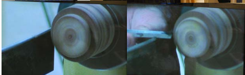
Turning a tenon on the end for the top was the first order of business.
