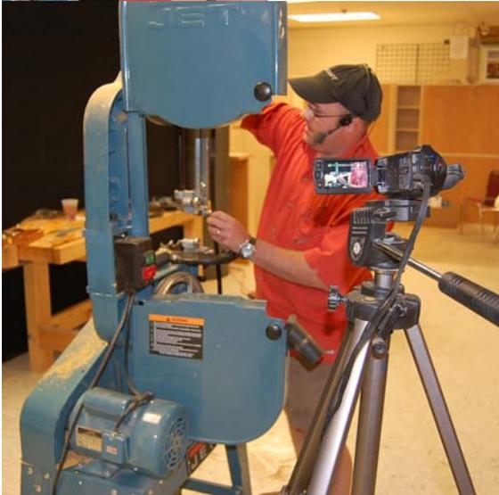
It is very important to make sure that the blade lines up properly because the blade's life will be shorted if not.
