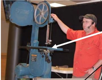
When working on the saw, it is easier to remove the table first. Then give it a good brushing off, inspect the tires. If they are getting loose replace it - not very expensive.
