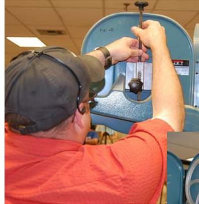
Some of the typical problems are vibration which can be caused by a bad belt or poor tires on the wheels.
