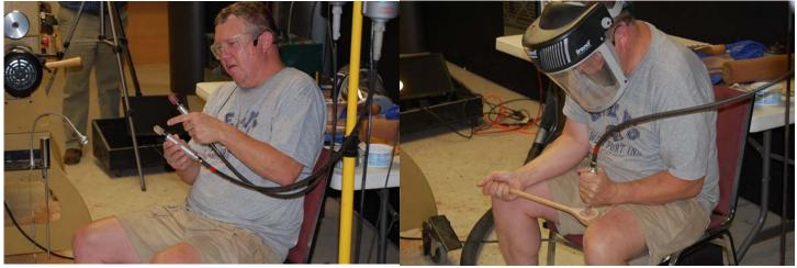
I think it's safe to say that the power grinding part of the demonstration had many on the edge of their seats, for more reasons than one. The process placed the work in close proximity to rather significant body parts but he explained the safety procedures he uses which included using tools that are not very aggressive, holding it properly, and using appropriate breathing and eye protection.
