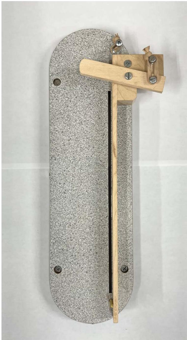
The Table Saw Blade Insert is modified by drilling three holes in it.
