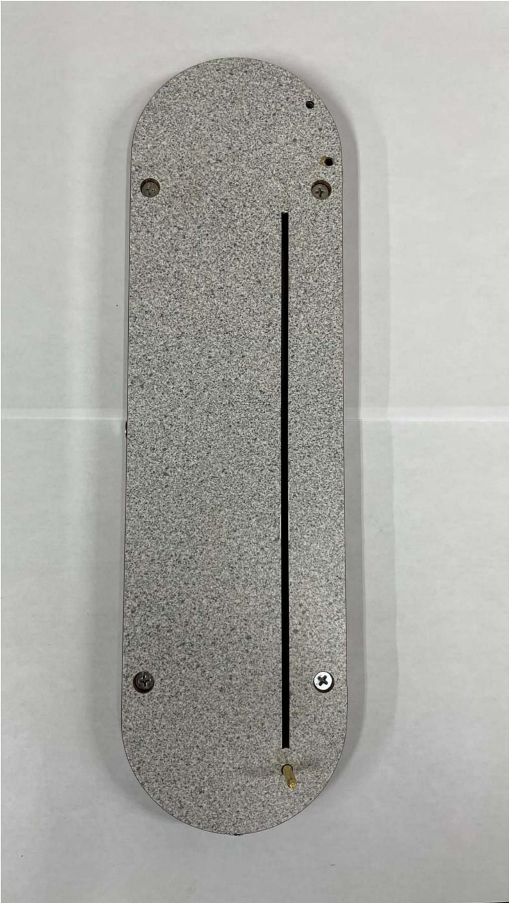
These are the screw hole locations for the Segment Flipper block mounting screw and the flipper return rubber-band screw. The holes are drilled a bit smaller than the thread diameter. The screws tap themselves into the blade insert. The location of the Segment Flipper block allows about 1/16" clearance to the saw blade. The hole locations are referenced to the upper-right corner of the blade slot.
