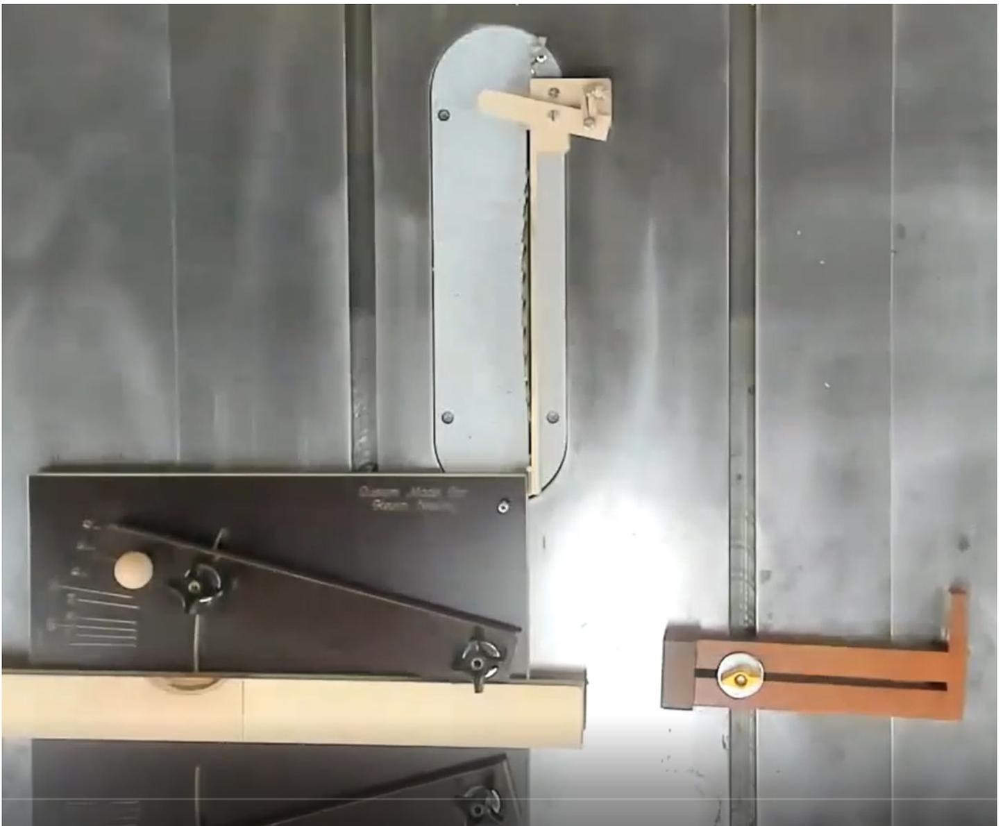
The Segment Flipper is constructed on a Leecraft DL-1 Zero Clearance Table Saw Insert so the insert and flipper can be easily removed and replaced with a regular blade insert. The DL-1 insert is made for Delta and other saws with a 3-3/4" x 13-3/8" opening, The flipper has about 1/16" clearance to the sawblade. The sawblade clearance is set by the location of the brass flipper pin at the bottom of the flipper and by the location of the flipper block's countersink screw hole.
