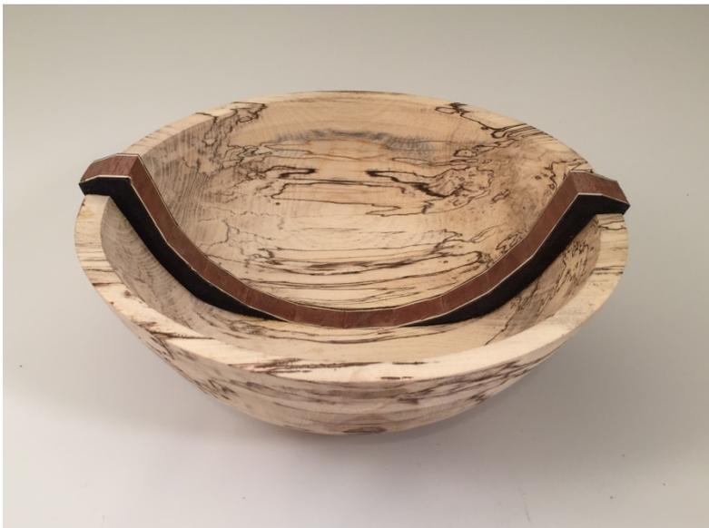
A little bit of veneer was glued to the segmented half-ring to dress it up. The hackberry blank halves and segmented half-ring were glued together.
