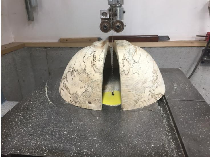
The hackberry blank was cut into halves on a bandsaw, through the long side of the blank. The rough cut surface was flattened on a belt sander.
