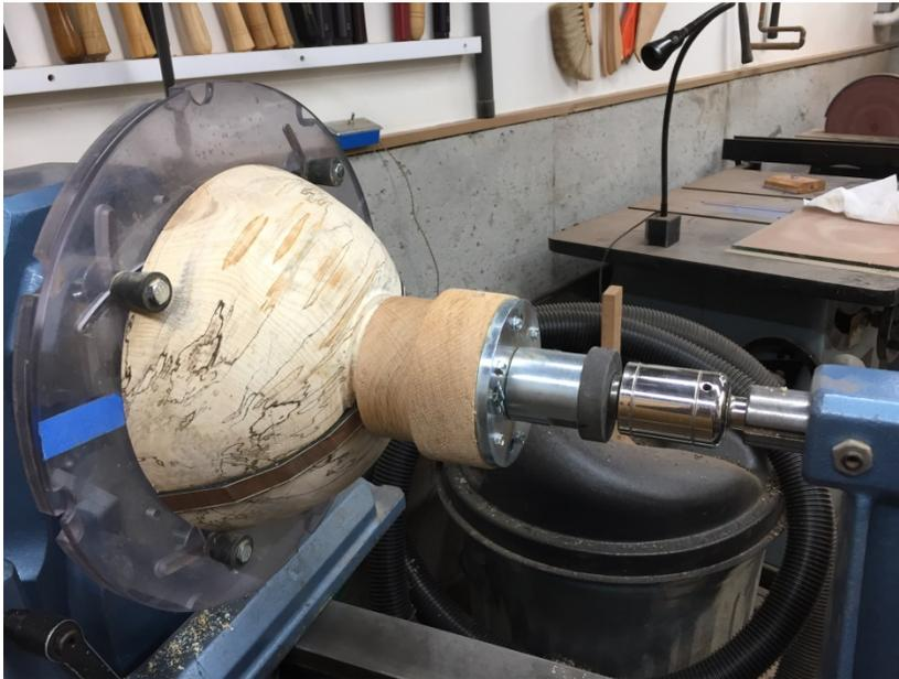
The bowl was glued to a faceplate with waste blocks and turned on a Vicmarc wood lathe.
