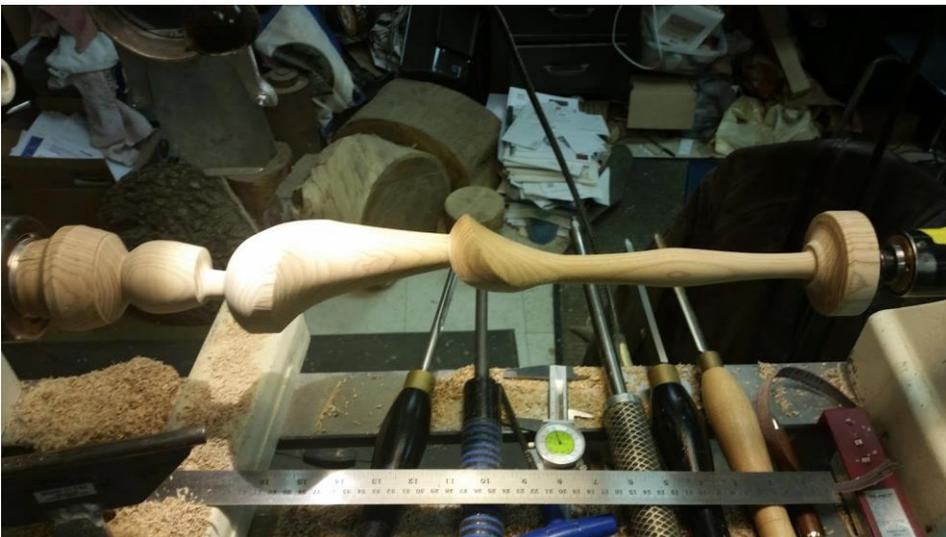
It's often useful to place a black posterboard beneath the turning in order to better see the eccentric horizon to be turned. The edge of the revolving axis will appear as a blur. Light cuts are helpful here. There
